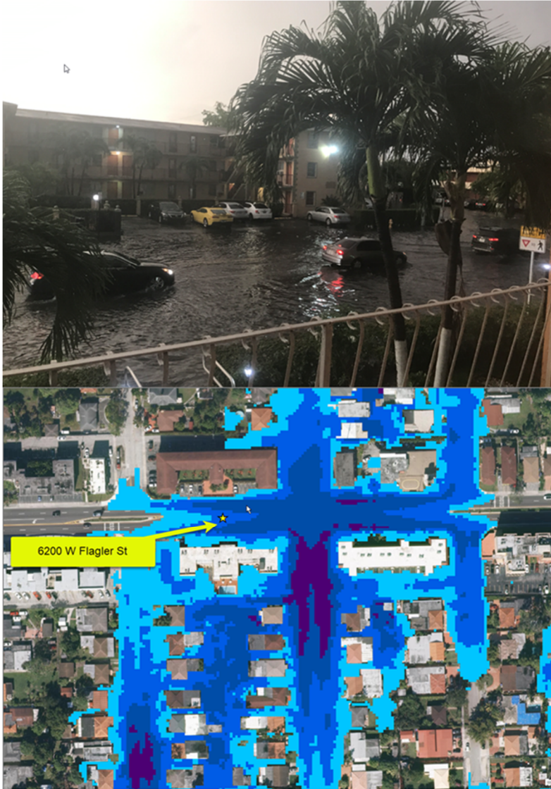
Figure A-20 Flooding Near S.W. 62 nd Ave at Renedo Apt. Building. and Model Prediction
