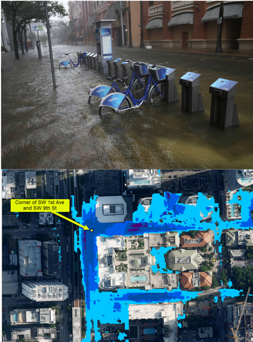
Figure A-13 Flooding Near S.W. 1 st Ave. and S.W. 9 th St. and Model Prediction
