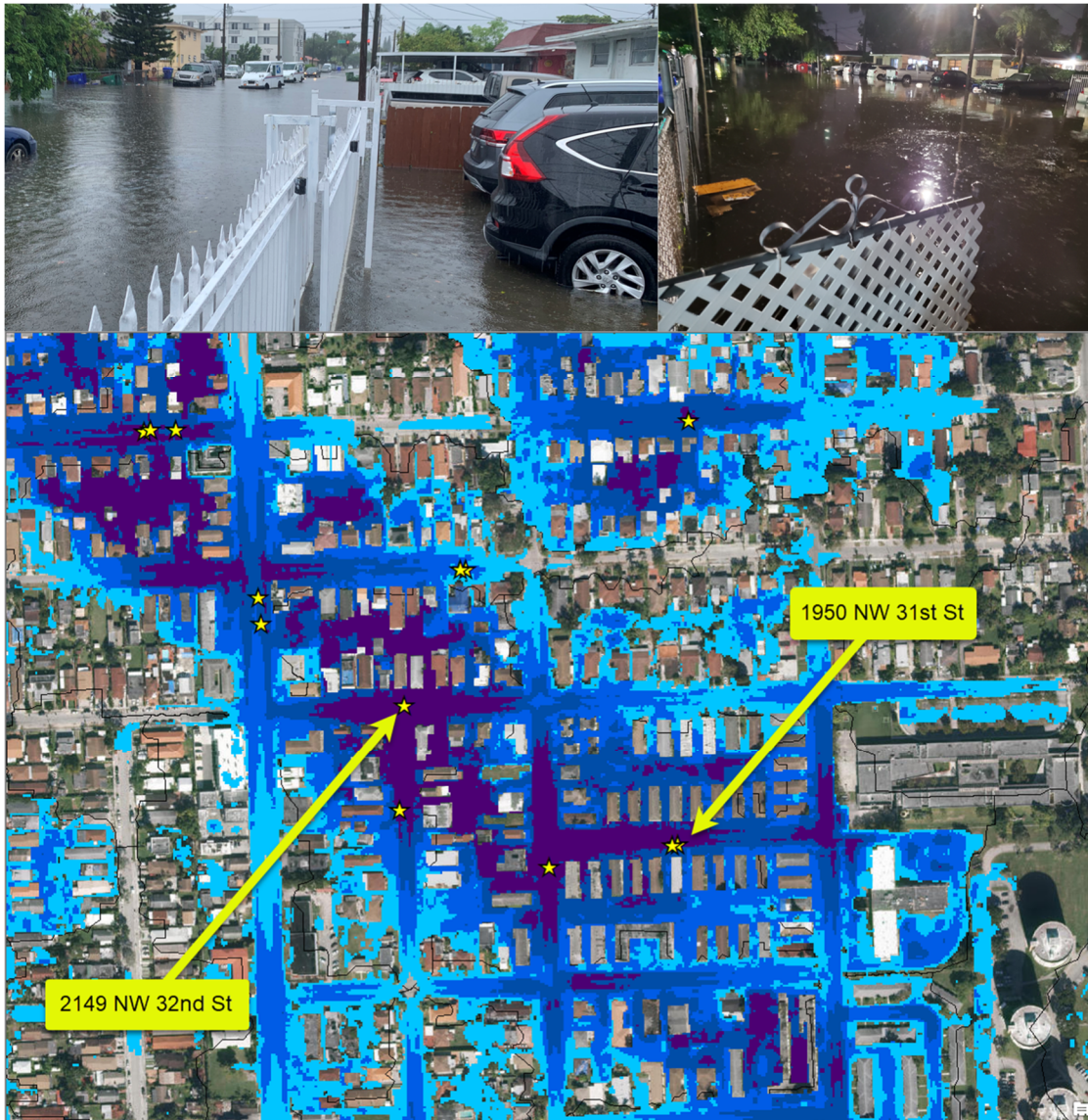
Figure A-17 Flooding Near N.W. 32 nd St. at N.W. 22 nd Ave. and Model Prediction
