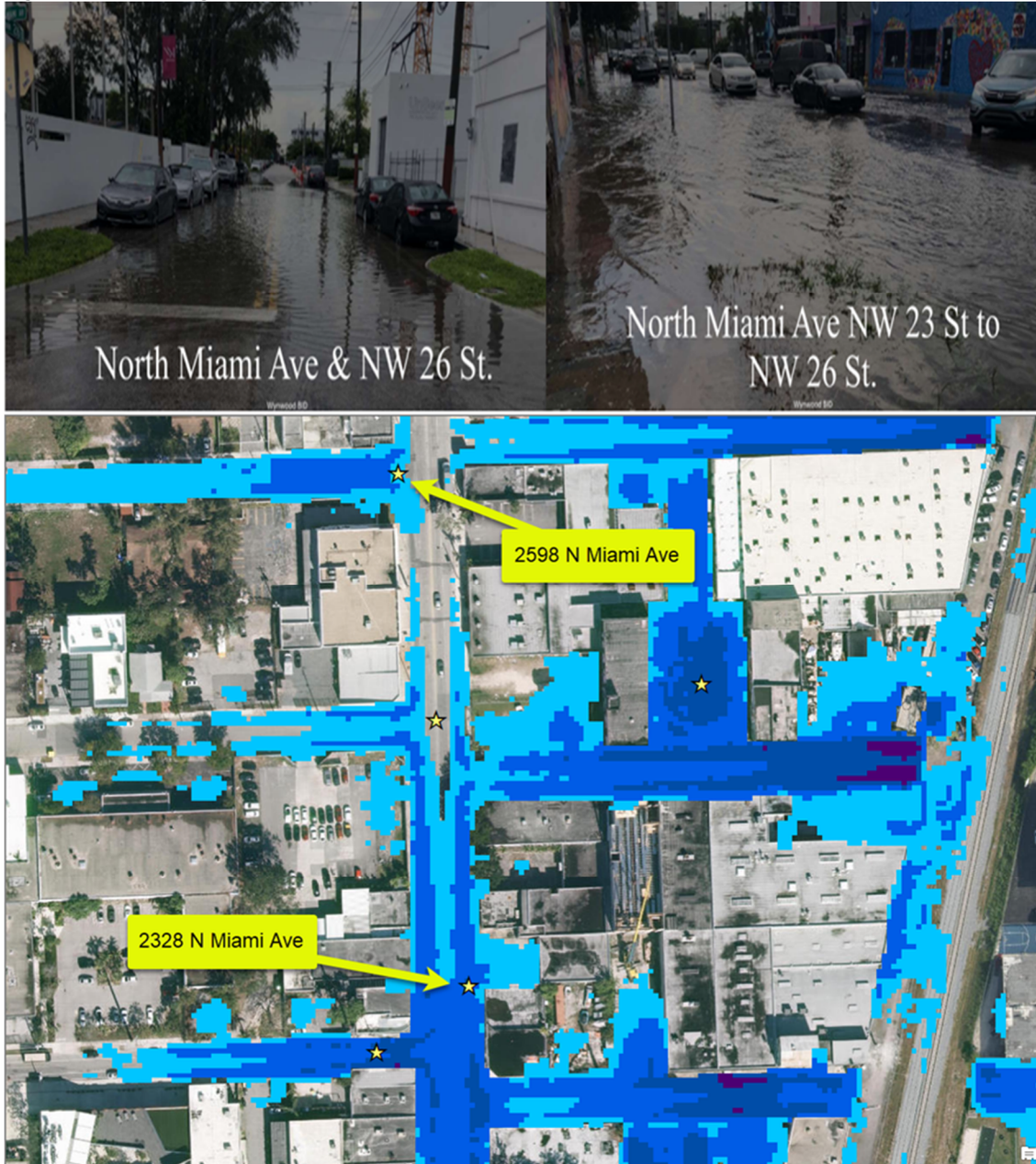
Figure A-7 Flooding Near North Miami Avenue between NW 26 St and NW 23 St and Model Prediction
