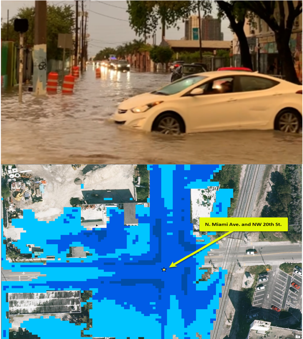
Figure A-8 Flooding Near North Miami Avenue at N.W. 20 th Street and Model Prediction
