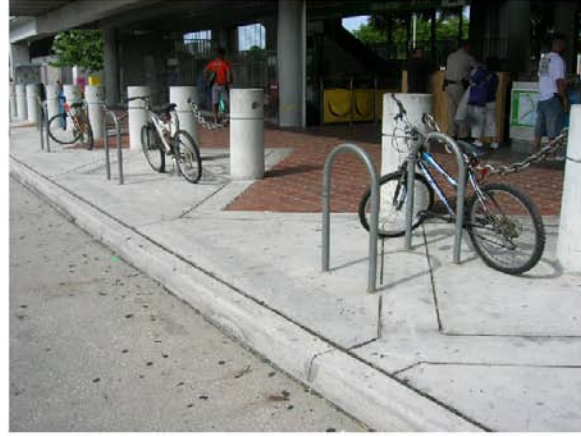
Inverted "U" Racks provide parking at the Allapattah Metrorail Station
