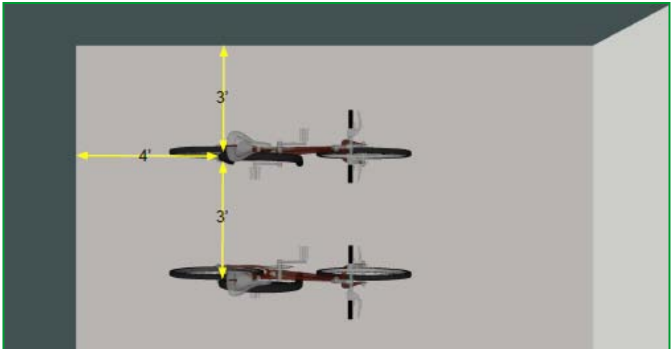
Figure 7- 18: Accessibility and Maneuverability Dimensions for Bicycle Parking Located Near Indoor or Outdoor Walls
